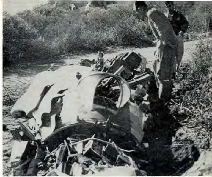
Strange are the happenings in an aircraft accident. Above, the nose section, cockpit and part of main fuselage section, while damaged heavily, are intact. Below, tail section, widely apart from wreckage, also was fairly well intact. Wings were found in another area; one barely damaged, the other amazingly good, considering this accident.
